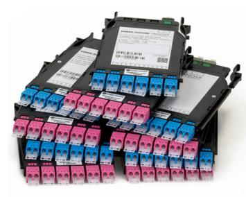
IANOS transition modules are built using fiber optic assembly, which transitions the MTP female at the rear side inside of the module to the LC duplex on the front side. Transition modules are used to build various plugand-play structured cabling permanent links.
